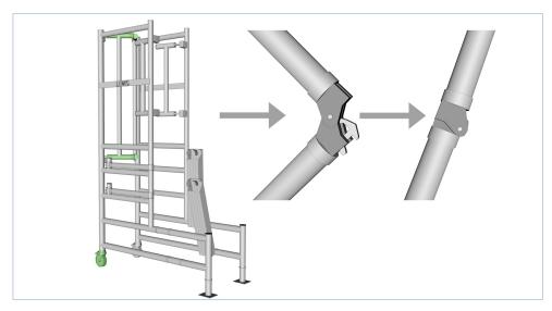
3. Place the steps securely on to the podium frame. Ensuring they are down and on securely
