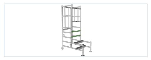
5. Place the podium platform at the chosen height, and safely lock into place the wind locks
